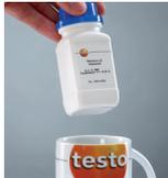
Remove the reference oil from the hot water. Do not let the oil come in contact with water!
