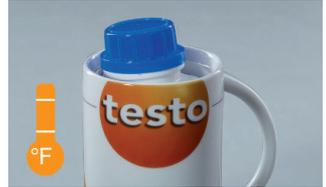
Before calibration or adjustment, warm the reference oil to approximately 122 °F in hot water.
