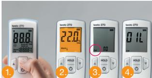
1. Press [Hold] for 2 seconds immediately after switching the instrument on.
