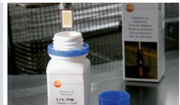
For accurate instrument testing, correction, or implausible measurements, we recommend calibration or adjustment with the Testo reference oil.
