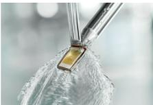
Clean instrument with mild detergent. Rinse sensor under running water and dry carefully with a soft paper towel.
