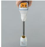
Immerse the sensor in the reference oil. The display will light up orange.
