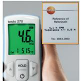
End the measurement as soon as the display lights up green. Compare value with label value from reference oil bottle:
