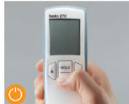
Switch the instrument on [ON].
